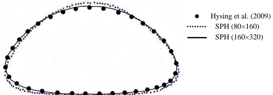
Fig. 6. The shape of the bubble at t=3 compared with FEM results of Hysing et al. [31].
